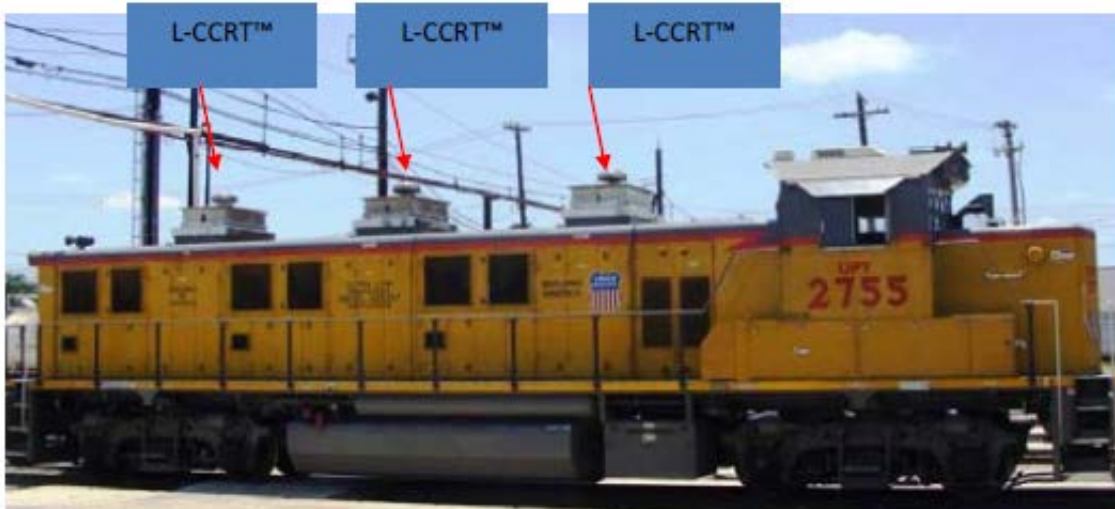
Passive DPF Locomotive Retrofit in California
