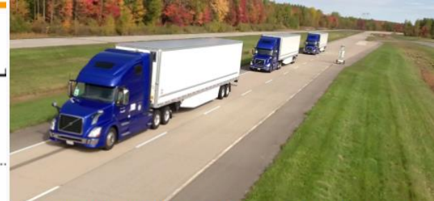
Three tractor-trailers travelling in close proximity to form a platoon during testing at Transport Canada's Motor Vehicle Test Centre
